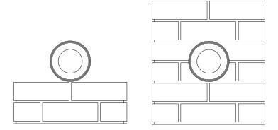
Build up brick work to desired height and set paper ring in place Complete remaining brickwork
